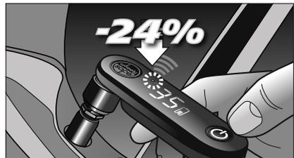
If the calibrated pressure has fallen below 24% the Sensor Reader will flash and bleep.
